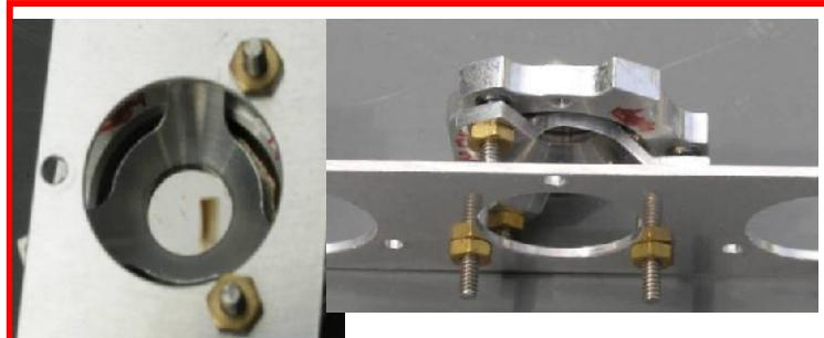
Differential Plunger for angles  $\neq 0^\circ$
