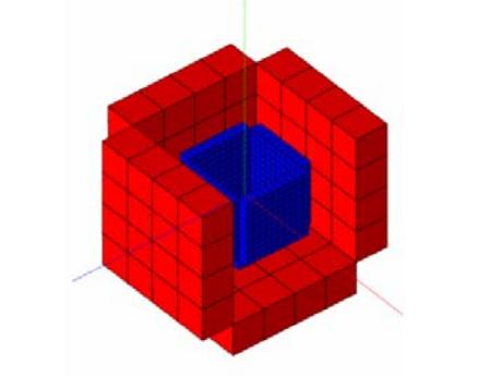
A 3D perspective view of a cube-shaped detector array. The outer edges of the cube are composed of red rectangular blocks. Inside this red shell, there is a single blue rectangular block positioned in the center. The entire assembly is set against a white background with three small coordinate axes (green, blue, and red) extending from the bottom left corner of the cube.
